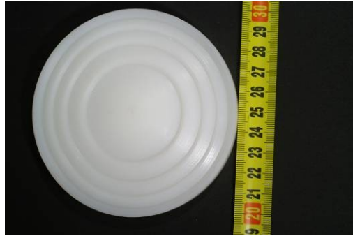
Figure 2: Plastic diffractive lens used in the experiment.
